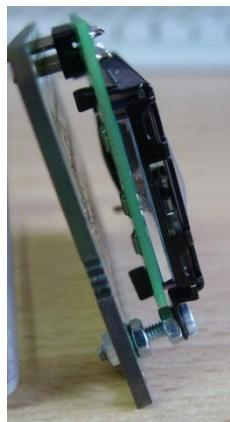
If the space available for the module integration is a bit short the depth of the sandwich may be reduced by 5-7 mm by directly soldering the LCD to the board, instead of using male and female headers. Please notice that if board removal is needed in the future, you will have to unsolder all pins from the LCD or the board.
