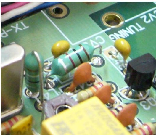
1) You will have to cut or lift one leg of L7 to remove the supply to the VXO. **It is not required to remove any part from the VXO!**
