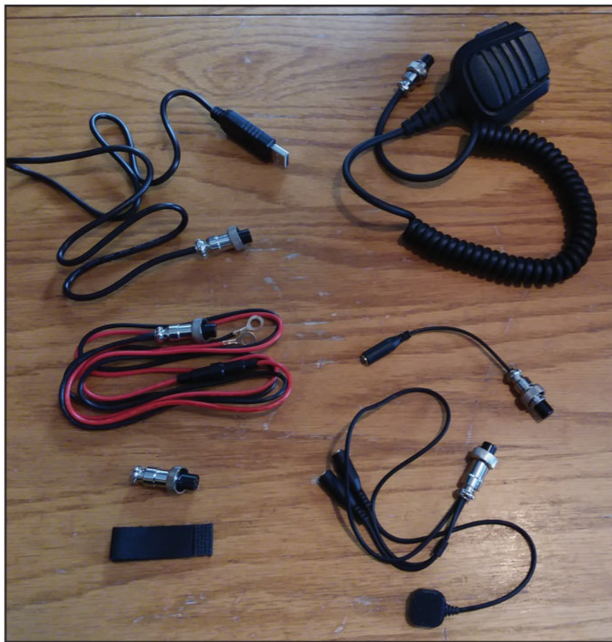
Photo C. Clockwise from top left: CAT cable for software updates, speaker / microphone, CW adapter (3.5-millimeter jack), headset, and mic adapter with PTT (3.5-millimeter jacks), Velcro® strap (for wrapping cords), GX-12 7-pin connector, and power cable for an external power source (9-15 volts).
