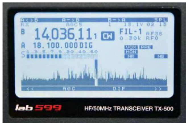
Figure 1 — The Lab599 TX-500 display conveys quite a bit of operating information at a glance, and even includes a spectrum scope. The wide vertical bar near the center of the scope shows the received bandwidth. Labels for the rows of soft keys above and below the display change depending on settings.
