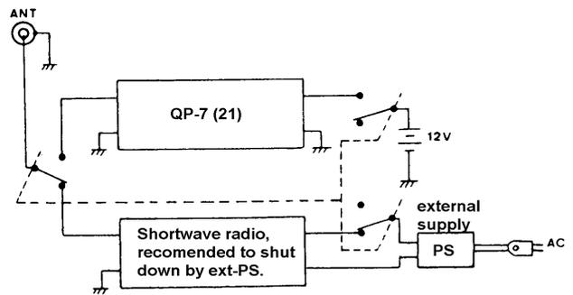
Figure 13. QP-7 Application AM transmitter with AF modulator.
