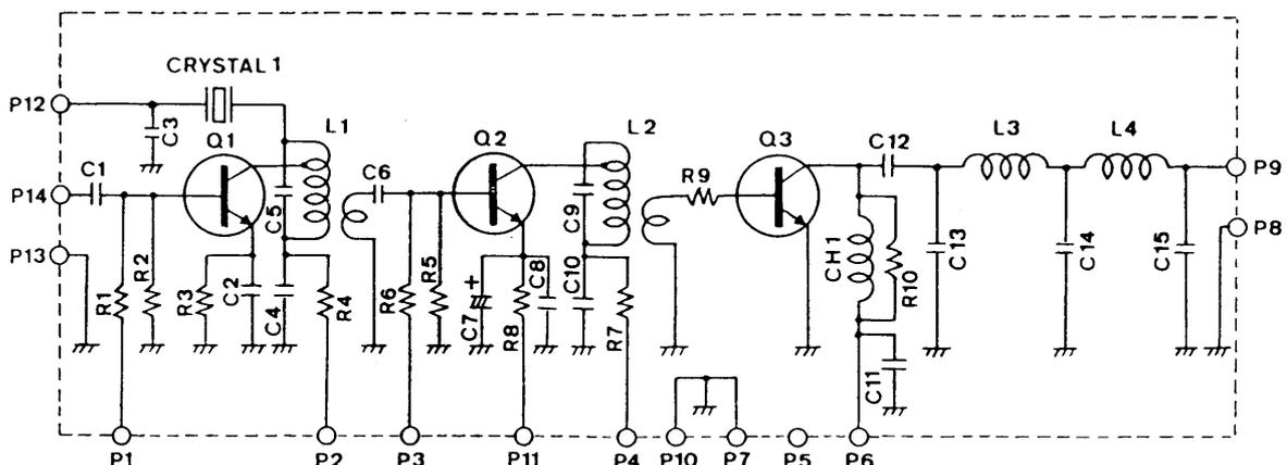
After you are done, place and solder the pins on the PCB. You may connect an ammeter to measure the supply current as shown in fig. 7. Without an ammeter, you must wire the pins, as shown in the dotted line in fig. 7. The transmitter will not function correctly, if you fail to wire the pins!
