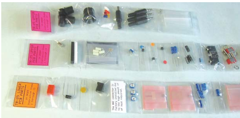
Figure 2 — The parts are packed in individual bubbles arranged in the order they are assembled. One set is for the lower board, another set for the upper board, and a third set for hardware and connectors.
