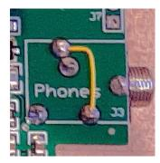
allow both headphone earpieces to play, **<u>but only if you</u>** <u>never intend to use a mono plug</u> connected to the "Phones" jack. To make this mod, the top case half must be removed by removing all the knobs and the four nuts holding the case half to the board assembly. Remove the four black case screws and lift off the upper-case half. Carefully solder in a jumper wire as shown in yellow in
