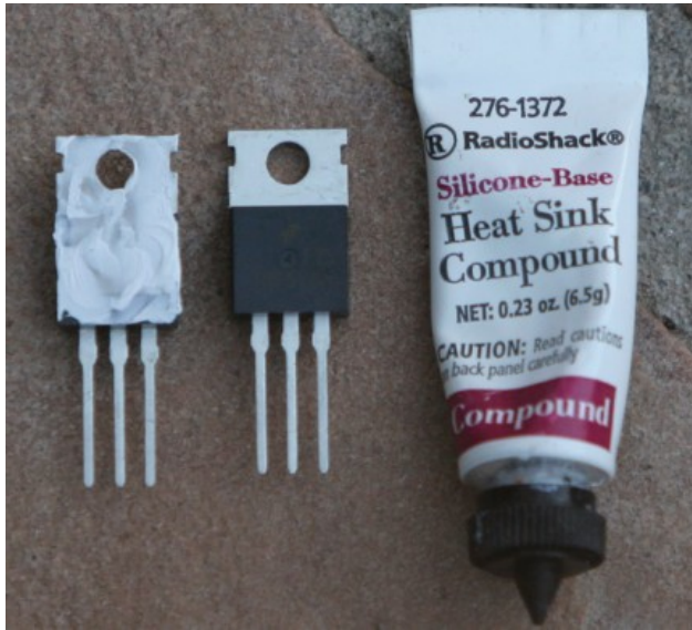
Figure 37. IRF510A transistors with heat sink compound applied to the back side
