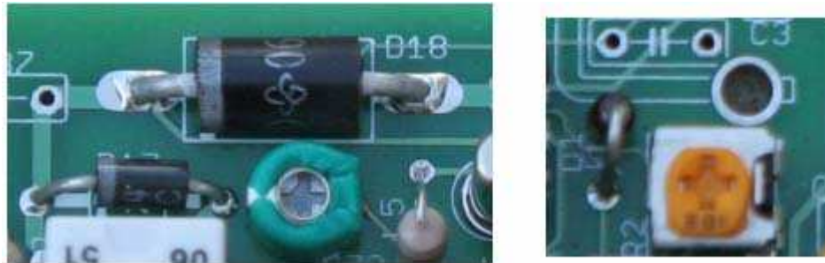
Illustration 1: D-17 and D-18 Installation (N7VE Photo)
