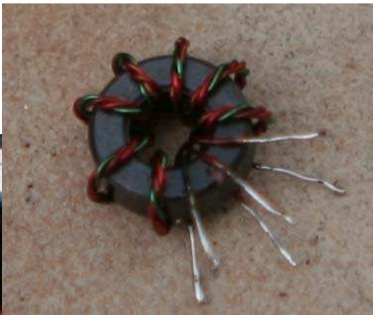
Illustration 20: T-2 Winding Detail (N7VE Photo)
