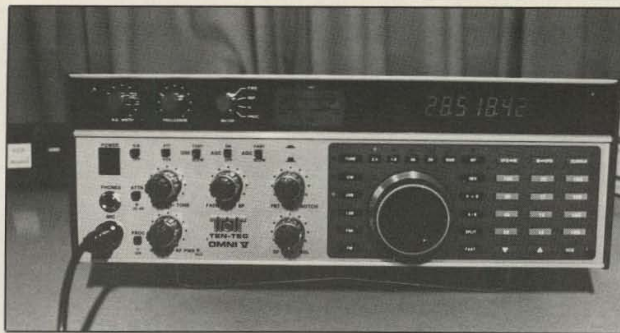
The front-panel layout of the Omni V is very well balanced with an easy-on-the-eyes frequency display, the analog controls on the left, and the large keypad around the main tuning control.
