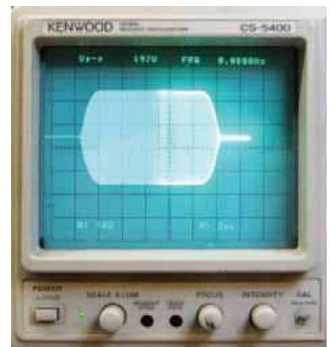
The CW keying waveform is quite acceptable, with rise and fall times of about 2ms.
