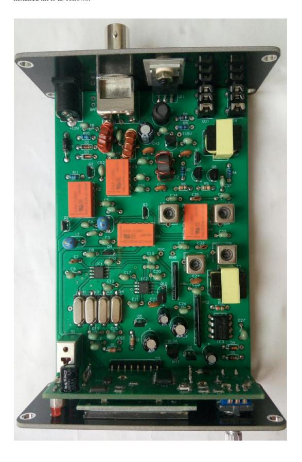
Now you can start debugging the kit. Check the installation and soldering, then turn on the power switch. If the current is about 50mA, it is normal. If the current is too large or too small, it indicates that there is a fault. After the subsequent debugging.
