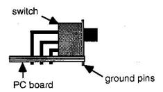
Remove the small metal tab (near the shaft) of the large potentiometer, R4. When you install R4, press it down into its PC board holes as far as it will go without forcing it. Solder R4.
