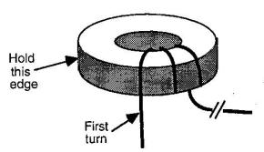
After winding, the turns should be spaced roughly even around most of the core, leaving a small gap between the first and last turns as shown below. (The number of turns shown in the drawing is different from the actual number of turns used.)
