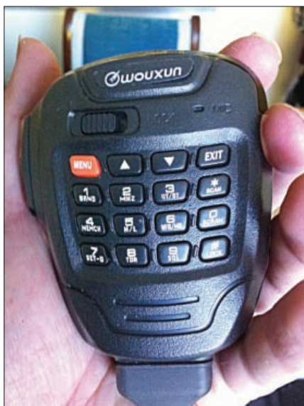
Unusually for a mobile transceiver the microphone supplied with the KG-UV920R is fitted with a small loudspeaker.
