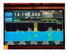
tory. The bandwidth displayed can be changed between either 50 or 100kHz and the main screen also shows an audio scope, which is useful, as well as SWR level, but this is not perfected yet on my version. More on this later.
