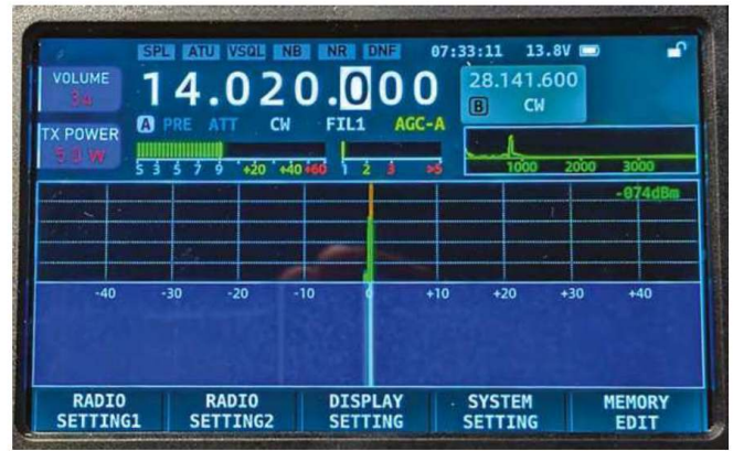
Figure 3 — The Xiegu X6100's 4-inch (800 × 480) high-resolution display.
