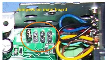
Jumpers on main board behind microphone socket
