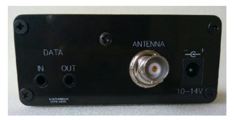
Power connection: Any DC power 10-14V, 1A connect to power jack.
