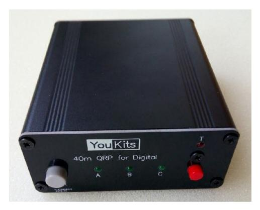
This 40m only Digital model QRP transceiver can work on FT8, FT4, JT65, PSK31 and SSTV etc connecting with computer(PAD) and related APP.
