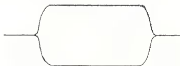
Fig. 3.—Keying Waveform of FL-50.
