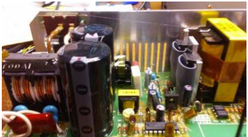
FT-1000MP switching power supply circuit board. Note slight bulges on the tops of the large capacitors.
