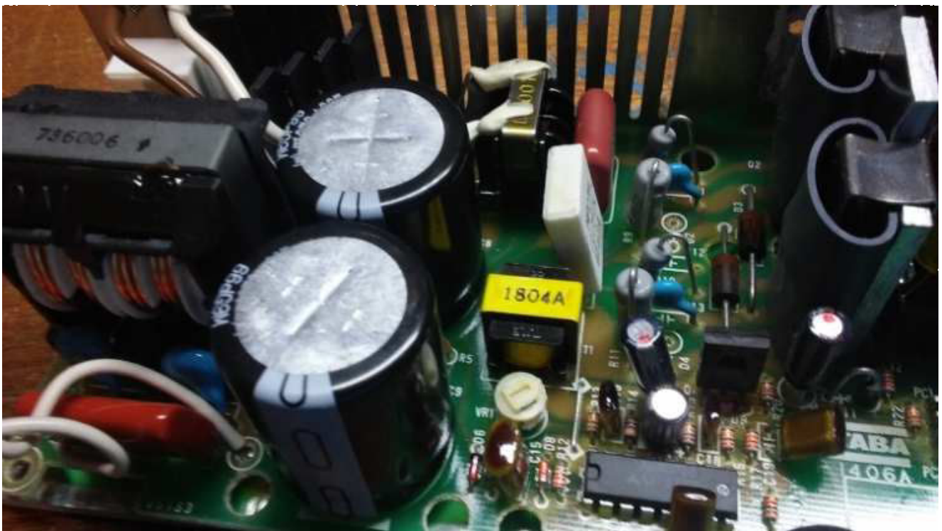
FT-1000MP switching power supply with new capacitors mounted.
