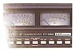
push-pull MRF422 final transistors, at 280 watts each, the transmitter training at 100 watts output. With 24V solled to the finals, transmitter thirder IMD is typically better than —40dB 14MHz, 100W out). Of course full remail and SWR protection is provided, and a cooling fan as standard and typical SWR.
