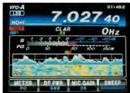
Figure 1 — The FT-991A's colorful touch-screen features a new real-time spectrum display. This view shows both a traditional spectrum scope (panadapter) and a waterfall display.
