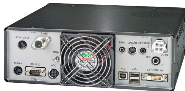
Figure 2 — The FTdx10 rear panel has connections for a variety of accessories. There is only one antenna jack, and no provision for a separate receive antenna. Note that the fan cycles on and off at slow speed in receive.
