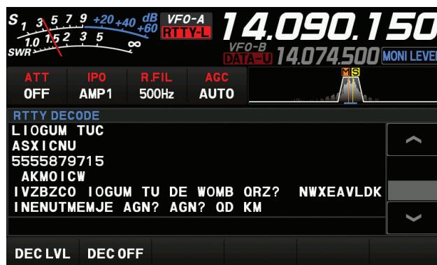
Figure 4 — During the BARTG RTTY Contest, the FTdx10's RTTY decoder tries to render readable text, but with mixed results. The passband display to the right of the AGC indicator shows mark and space frequencies to aid in tuning.
