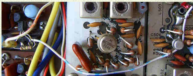
Insulated wire as "antenna" for the marker generator.
