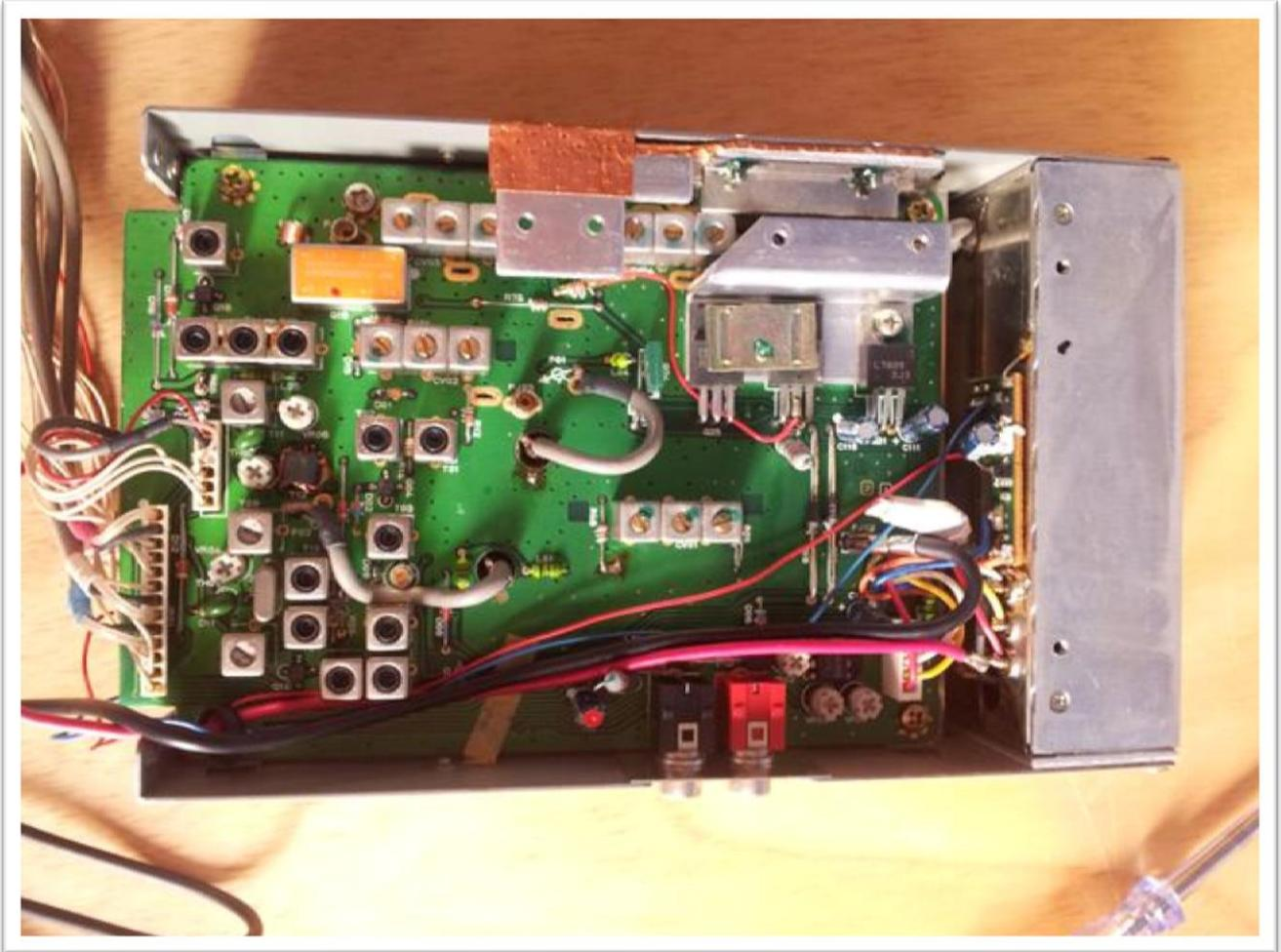
Apply some insulation tape to the old coax and fit the new coax.
