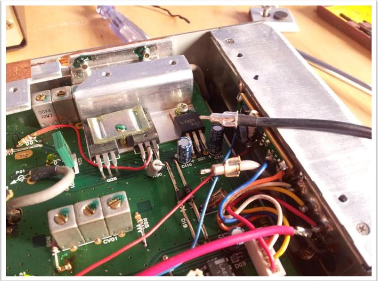
Remove the original coax and connect the new cable <sup>1</sup>
