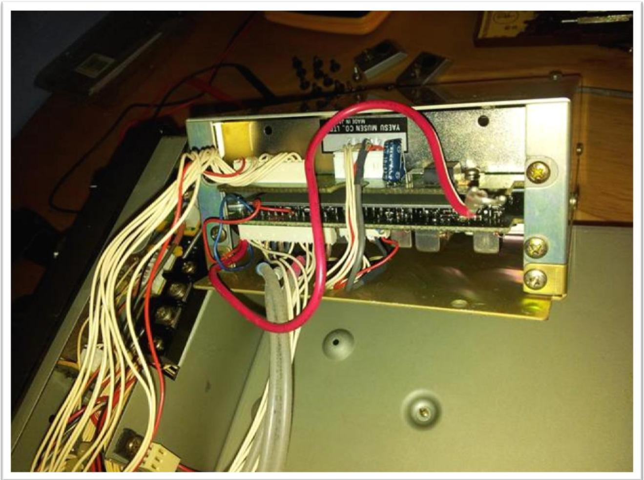
Open the radio and release the 1.2 module.
